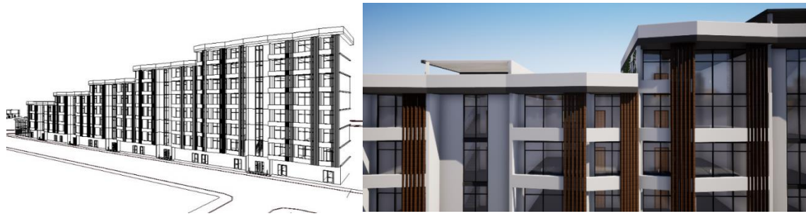
Fig. 5. Facade systems with vertical equipment solar panels
